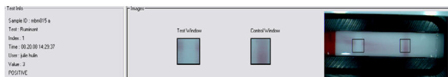
FIGURE 7 : FALSE POSITIVE RESULT (COLOURED STRIP WITH A WHITE TEST LINE)
